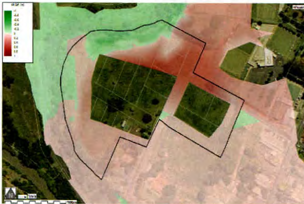
Figure 7 - Lowered riverside park + constructed channel, Flood level difference
